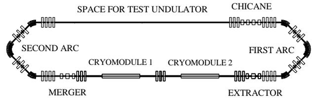
Figure 4: Lattice design of the test ERL.
