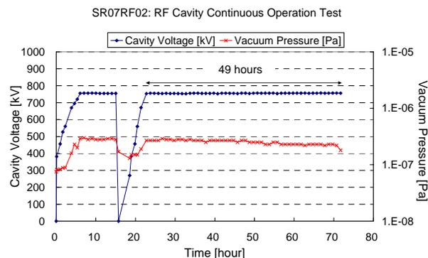
Figure 8: Result of the RF cavity continuous operation test for the station SR07RF02.
