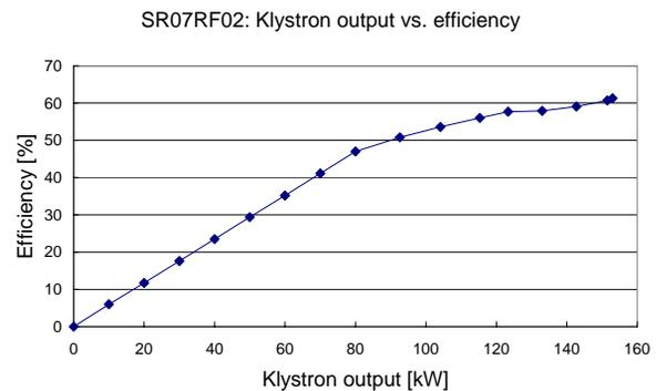
Figure 7: Result of the klystron efficiency measurement for the station SR07RF02.
