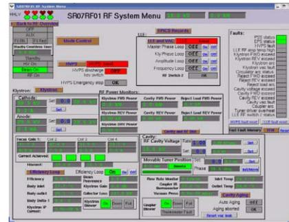
Figure 2: EPICS control screen of the single RF station.
