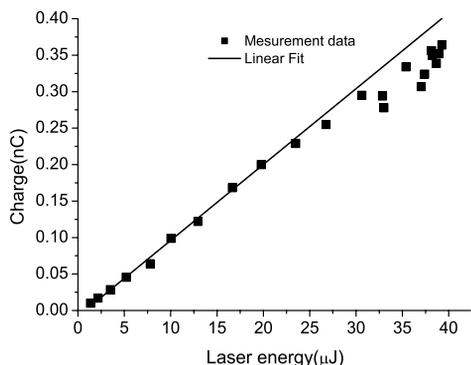
Figure 6: Charge versus laser pulse energy for the photocathode RF gun. The Max. RF field at cathode is about 75MV/m and injected RF phase is about 50°
