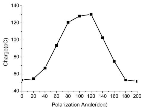
Figure 7: The charge measurement as a function of the laser polarization angle
