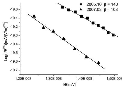
Figure 2: Fowler-Nordheim(F-N)plot for dark currents where  $E$  is the maximum gradient on the cathode and  $I$  is the Peak current. Square and triangle data are dark current with different RF conditioning time about 200 hours and 250 hours, respectively.
