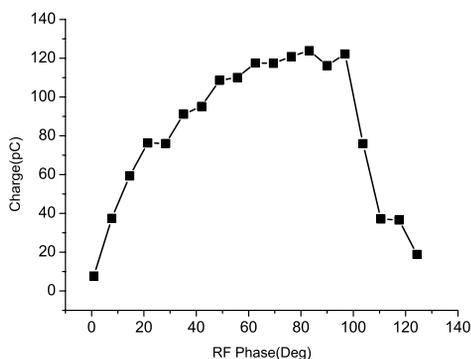
Figure 5: Photoelectron charge vs RF gun phase
