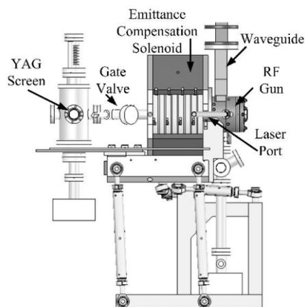
Figure 1: Layout of the photocathode RF Gun system.
