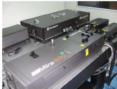
Figure 3: picture of laser system.
