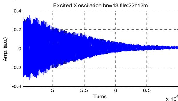
Figure 5: Horizontal damping process in HLS.
