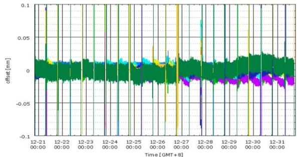
Figure 4: Vertical orbits at BPM during two weeks.
