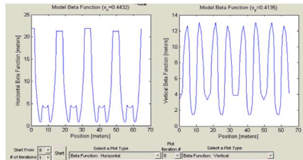
Figure 6:  $\beta$  functions of current operation mode of HLS.
