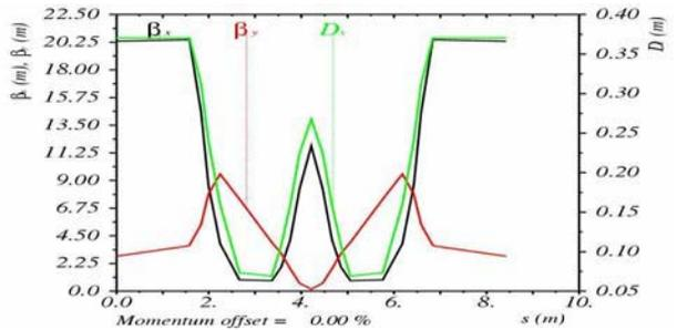
Figure 5: Beta and dispersion functions of one cell
