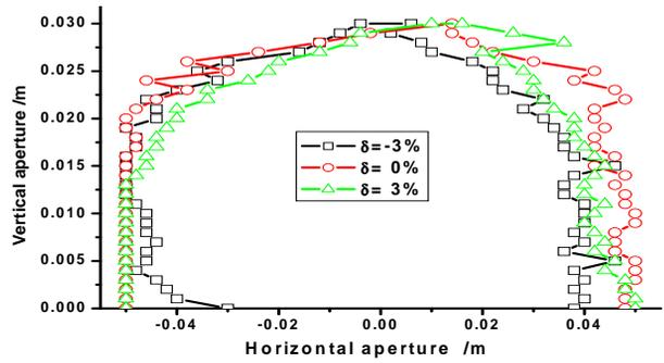
Figure 4: Dynamic aperture for mode A
