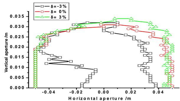
Figure 6: Dynamic aperture for mode B
