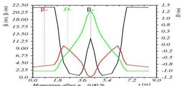
Figure 7: Beta and dispersion functions of one cell
