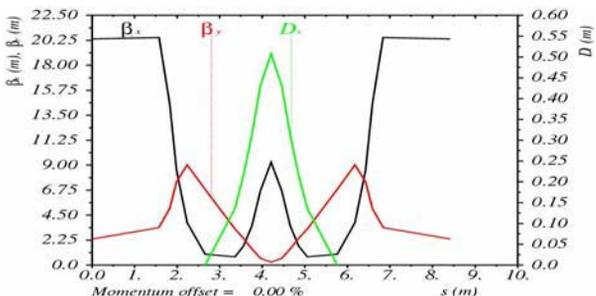
Figure 3: Beta and dispersion functions of one cell
