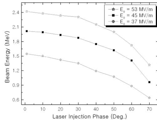
Figure 4: The beam energy as a function of the laser injection phase with different field gradients.
