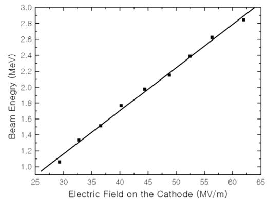
Figure 5: The beam energy as a function of the field gradient in the RF gun.
