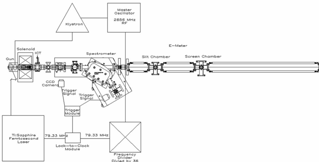
Figure 3: Schematic diagram of the gun test stand (GTS) at the PAL. The GTS consists of 1.6-cell PC RF gun with emittance compensation solenoid, a Ti:Sa femto-second laser, a spectrometer, and an E-Meter.
