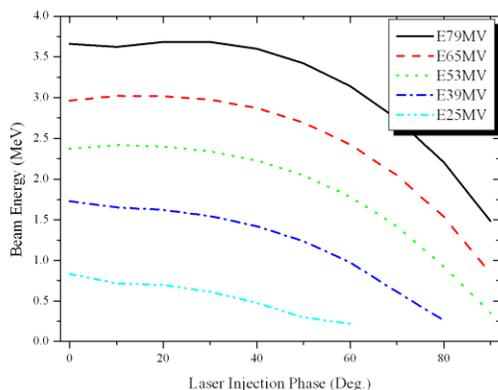
Figure 2: The beam energy simulation as a function of the laser injection phase with various electric fields in the cavity.
