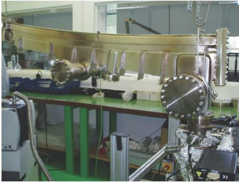
Figure 2: Prototype of the Bending vacuum chamber in the test stand.
