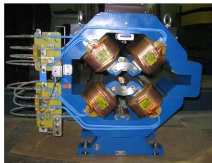
Figure 1: SR Quadrupole with a side opening to let a beamline pass through.
