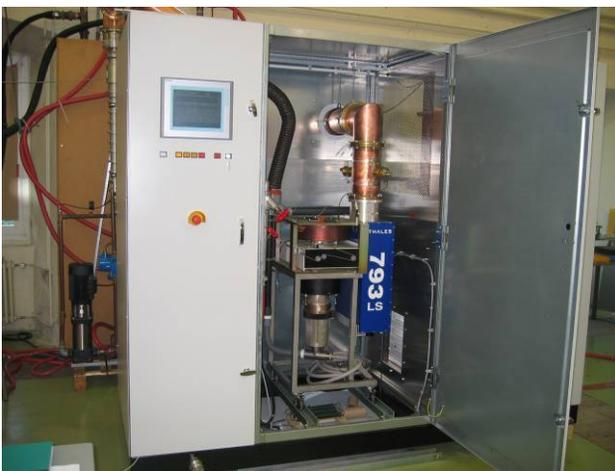
Figure 3: IOT under test.
