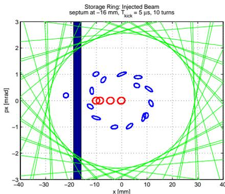
Figure 6: Injected (blue) and stored beam (red) in the horizontal transverse phase space at the injection point. The blue region corresponds to the septum location, the green lines give the physical aperture all along the ring.
