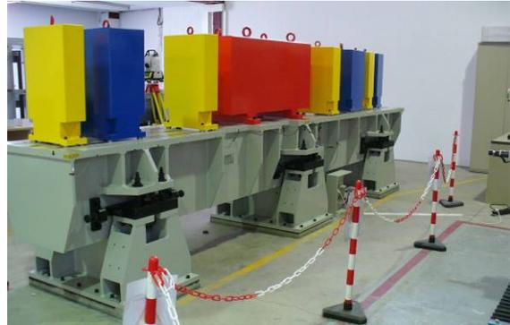
Figure 4: SR girder prototype with dummy magnets.
