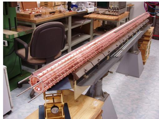
Figure 5: Accelerating structure before brazing.
