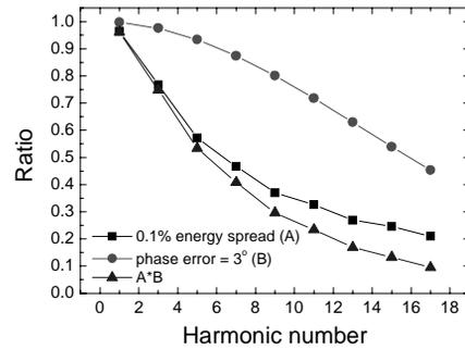
Figure 7: Flux decrease ratio as a function of the harmonic number under a phase error 3 deg, energy spread 0.1%, and the combination factor of phase error 3 deg and energy spread 0.1%.
