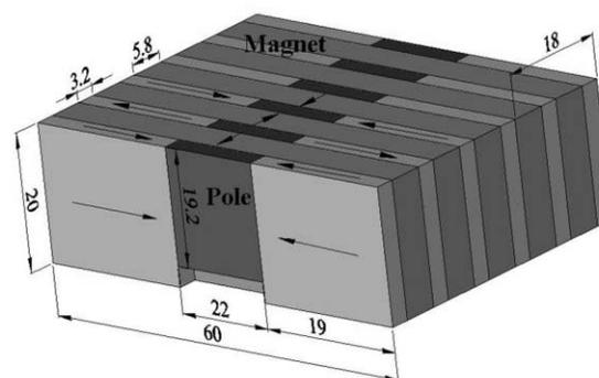
Figure 2: Schematic drawing of the magnet array of the cryogenic permanent-magnet undulator.
