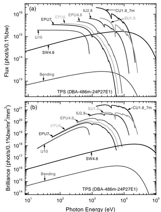
Figure 1: The spectrum of (a) flux and (b) brilliance at the TPS insertion devices for which the spectrum was calculated depends on parameters in Table I except the length of CU1.8.
