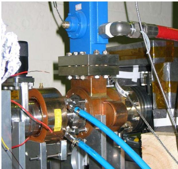
Figure 2: The thermionic cathode rf gun has been installed in the test stand for high power processing and preliminary beam test
