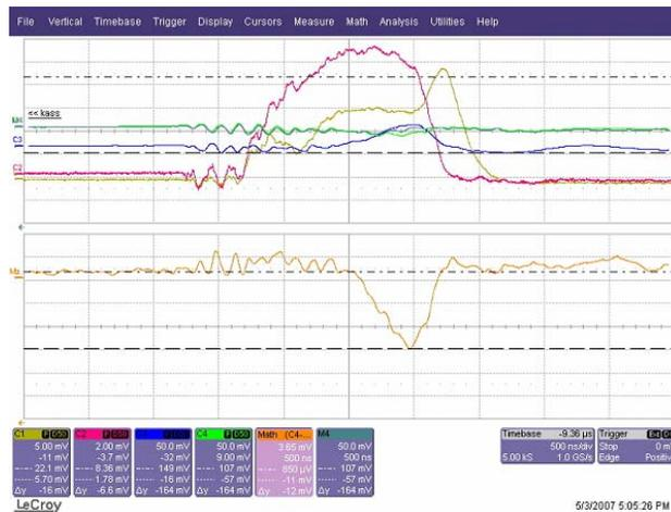
Figure 3: Observed cavity forward power (red), reverse power (yellow) and dark current (orange) signals at 4 MW cavity forward power during high power processing.
