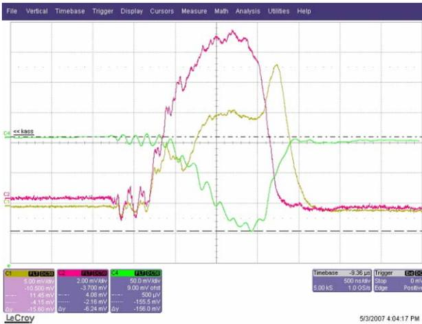
Figure 4: Observed cavity forward power (red), reverse power (yellow) and dark current (green) signals with cathode heater turned on.
