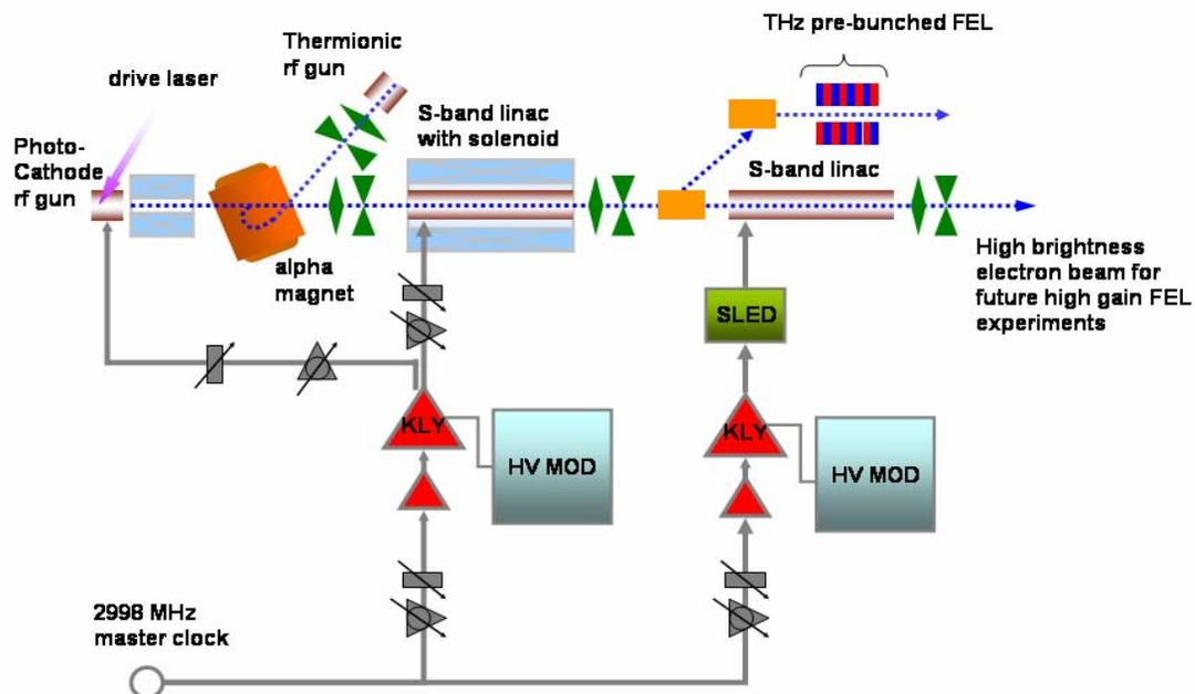
Figure 1: Schematics of the NSRRC high brightness injector
