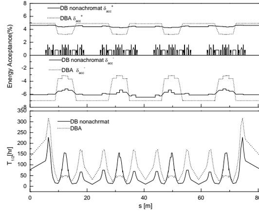
Figure 2: Energy acceptance and Touschek lifetime results along a super-period for DB in achromat and nonachromat mode.
