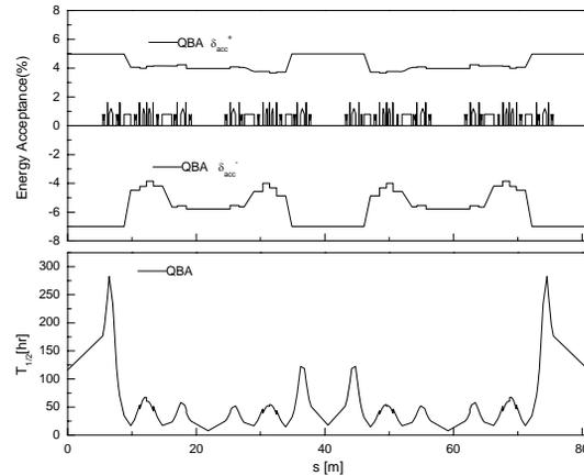
Figure 3: Energy acceptance and Touschek lifetime results along a super-period for QBA.
