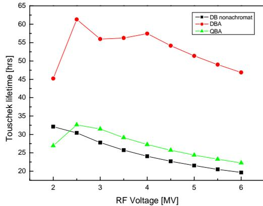
Figure 4: Tauschek lifetime as a function of RF voltage.
