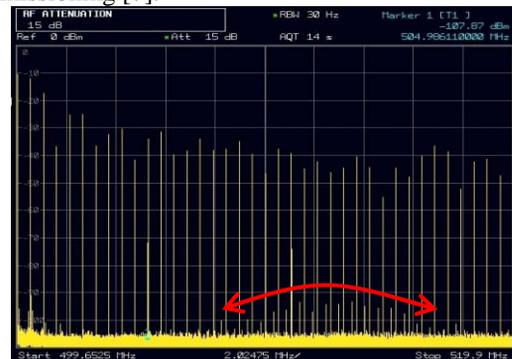
Fig. 2: Spectrum Analyser traces for 150 mA, 2/3 fill, chromaticity +2 in both planes, showing the prevalence of ion related induced instabilities over the Resistive Wall.
