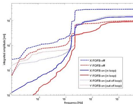
Fig. 5: Results of FOFB tests during commissioning.
