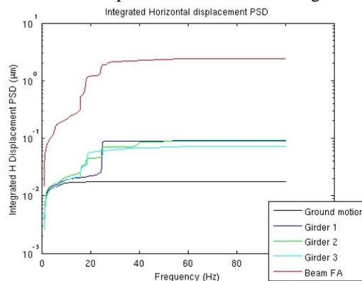
Fig. 4: Horizontal PSD comparison of ground motion with vibration of the three girders and beam motion.
