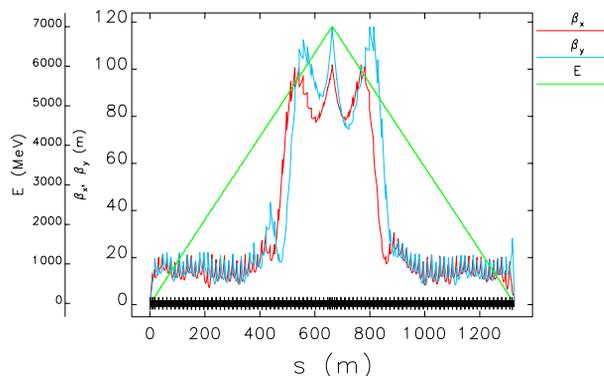
Figure 3: Doublet optics for the 10 MeV to 7 GeV linac, showing lattice functions for acceleration and deceleration.
