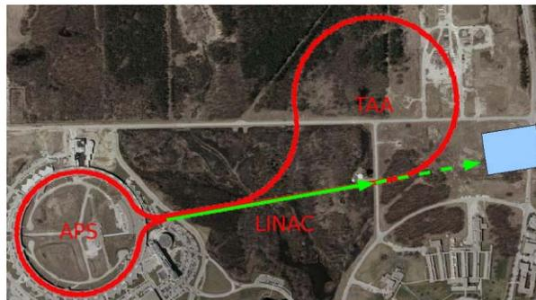
Figure 1: Diagram of the ERL concept, showing the APS itself, the linac, and the turn-around arc (TAA). The ERL path is from elegant’s floor coordinate output.
