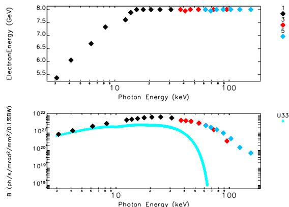
Figure 6: Results of optimization of beam energy and undulator period to maximize the brightness at various target photon energies for various undulator harmonics (1,3,5). Results for U33 at 7 GeV are shown for comparison.
