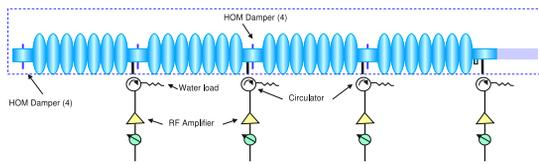
Figure 2: Cryomodule concept using nine-cell cavities.
