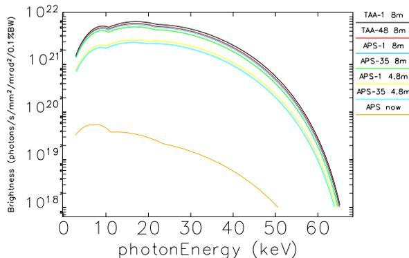
Figure 5: Comparison to present brightness using U33 undulators of various lengths in various positions in the ERL.
