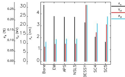
Figure 2: Results for 14.4 m of various wigglers for the APS low-emittance zero-dispersion lattice.
