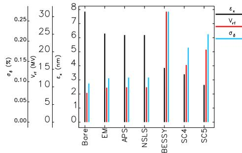
Figure 1: Results for 14.4 m of various wigglers for the APS high-emittance zero-dispersion lattice.
