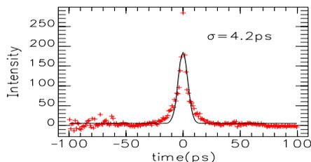
Figure 3: The average length of the slitted pulse when the time jitter is removed.
