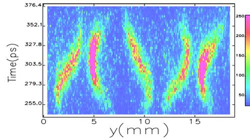
Figure 1: The side views of a bunch at turn 63 to 67 after a vertical kick.
