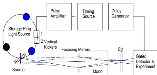
Figure 4: The short-pulse generation scheme.
