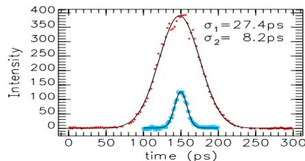
Figure 2: The length of the long-time-overlapped pulses. Red crosses, without the slit; blue squares, with the slit.
