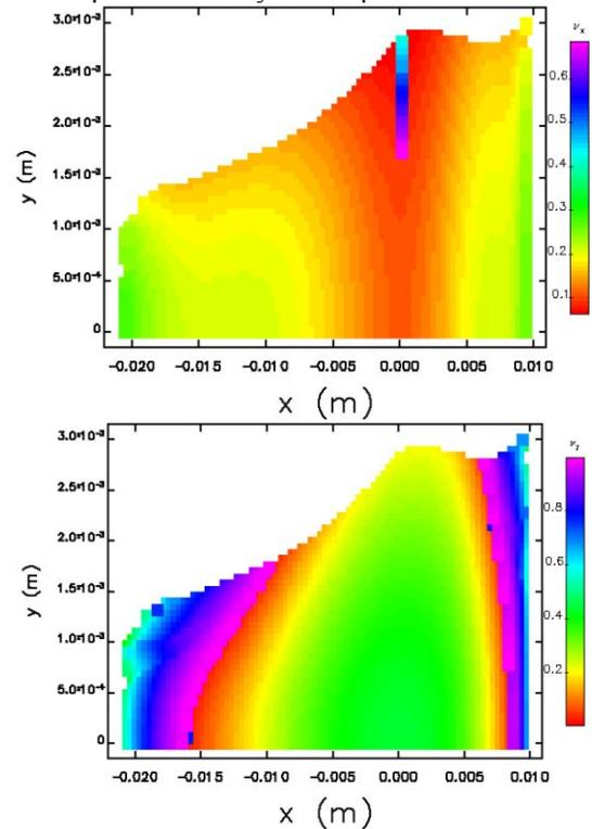
Figure 3: Dynamic aperture of ideal lattice with optimized sextupoles. Colors show betatron tunes, top – horizontal betatron tune, bottom – vertical betatron tune.
