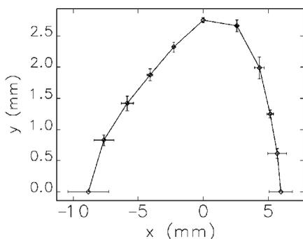
Figure 5: Average dynamic aperture based on 100 random error sets. Error bars show rms variation of results.
