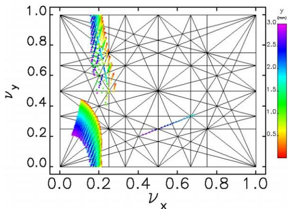
Figure 4: Tune diagram showing tune shift with vertical amplitude for the ideal lattice. Colors show vertical amplitude.
