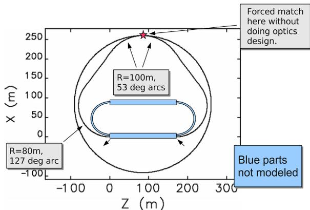
Figure 3: Layout of the infield ERL indicating parts modeled by elegant. At injection into the ring, detailed optics matching was not performed, but an ideal match was assumed for the emittance and energy spread calculations.
