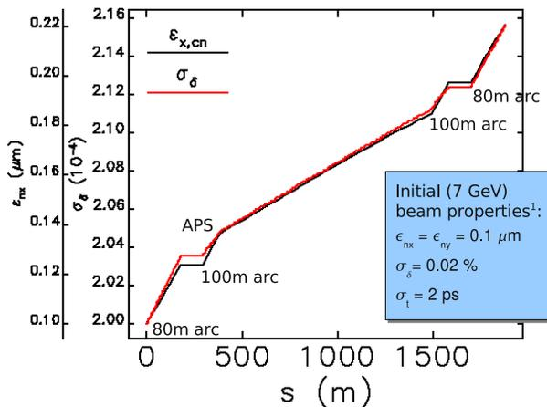
Figure 4: Emittance and energy spread increase calculated from the exit of the ERL linac at 7 GeV through the APS and back to the entrance of the ERL. The 80- and 100- m values refer to the mean radii of the bending arcs.
