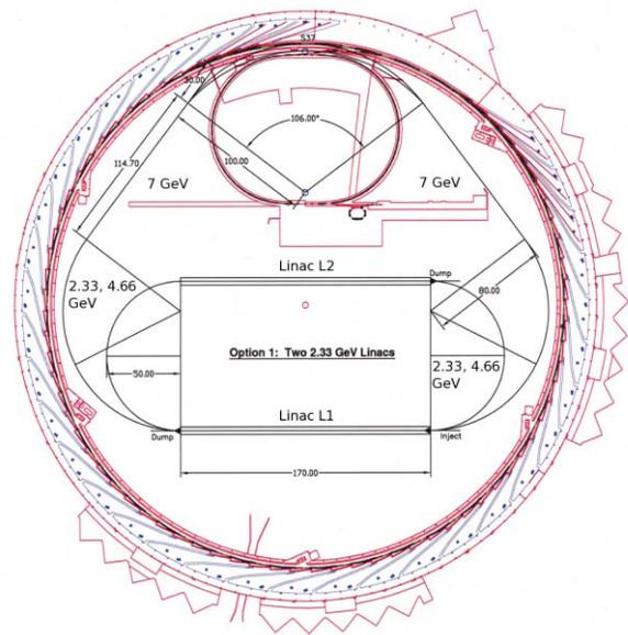
Figure 2: Layout of the three pass recirculating linac in the APS infield. Shown at each end of the linacs is a single arc which actually contains two beams of energy 2.33 and 4.66 GeV respectively.
