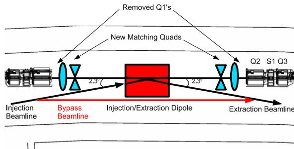
Figure 1: Storage ring sector 37 ERL injection and extraction configuration.
