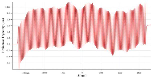
Figure 3: Trajectory in Hi-Tech's first-article undulator after tuning. The trajectory is straight to within 2 microns over the entire 3.4-m-long device.
