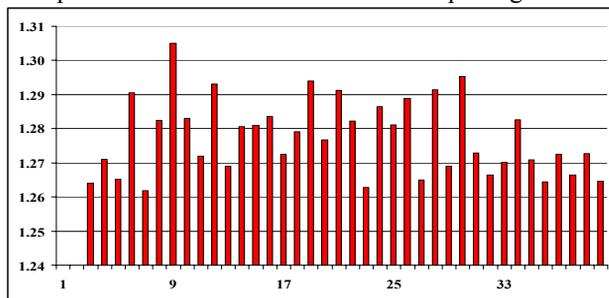
Figure 6: Measured average peak field for each undulator (3-40) at factory acceptance. All undulators will be tuned in the LCLS magnet measurement facility.
