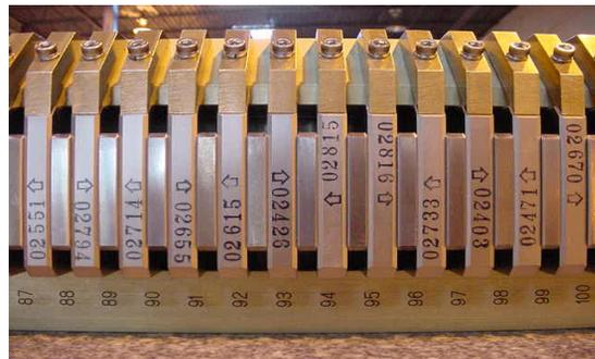
Figure 5: Verification photo from Metalex, showing slot numbers, magnet numbers, and magnet orientations.
