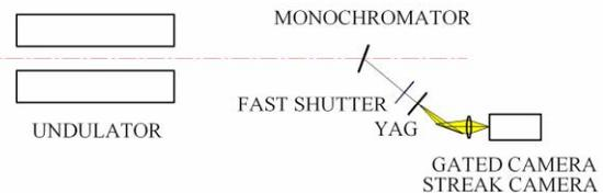
Figure 6: Optics arrangement for undulator-based fast imaging to detect beam motion / tilt outside of the zone.
