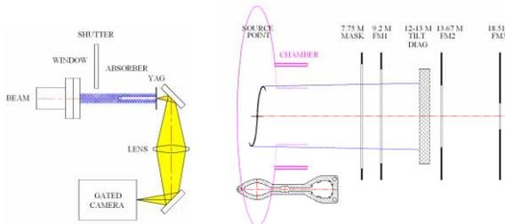
Figure 2: Left: schematics of a tilt diagnostic using a gated camera for snapshots of the tilted electron beam. Right: vertical aperture diagram of the beamline.
