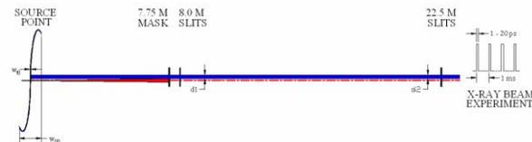
Figure 3: BM x-ray beamline in off-axis collimator mode.
