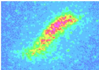
Figure 5: Visible light streak image of a tilted bunch [4].
