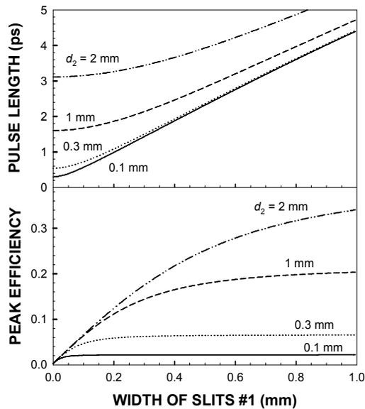
Figure 4: BM x-ray pulse length and peak flux efficiency.
