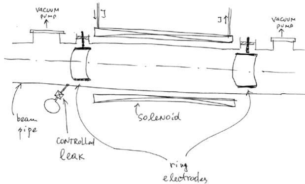
Figure 2: Layout of the electron column. .
