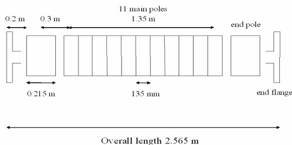
Figure 2: Schematic diagram of the MPW.
