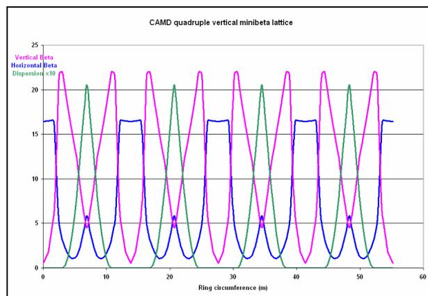
Figure 3: Lattice functions of an optic with a vertical minibeta in each of the 4 long straights.
