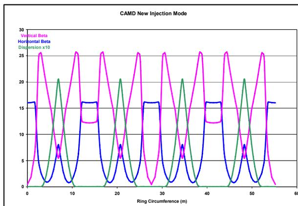
Figure 1: The lattice functions of the New Injection Mode.
