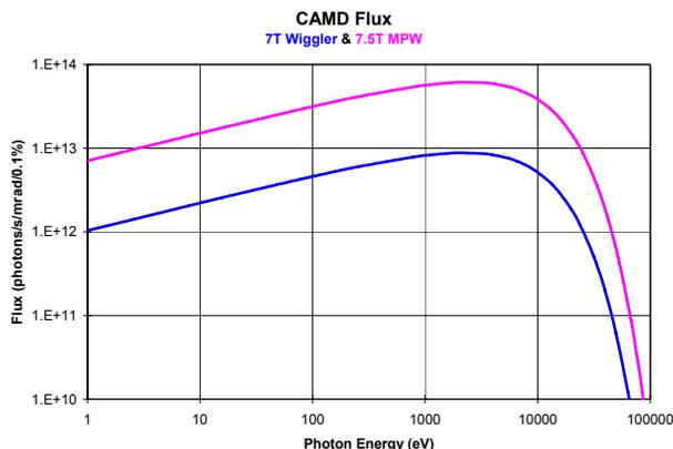
Figure 4: Flux spectrum from the 7.5 Tesla 11 pole MPW compared with the 7 Tesla wavelength shifter.
