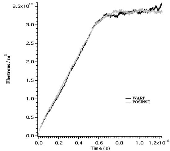
Figure 2. Electrons per  $\text{m}^3$  (averaged over 2.3 cm radius beampipe) vs time in ideal dipole from WARP-POSINST and POSINST.  $64 \times 64$  transverse grid.  $\Delta t = 5 \times 10^{-12}$  s.
