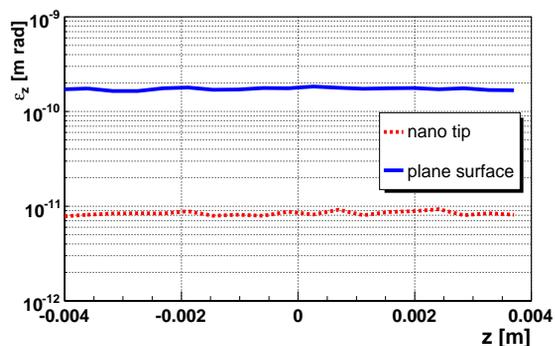
Figure 7: Final slice emittance distribution from the 10 nm nano-tip and from the 1  $\mu\text{m}$  plane surface.
