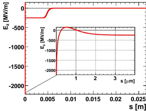
Figure 1: Longitudinal electric on axis field profiles, field near tip shown in the inset.
