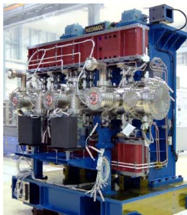
Figure 3: Picture of the first ALS in-vacuum undulator with 3 cm period and 1.52 T maximum field.
