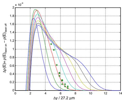
Figure 5: Measured femtosecond x-ray flux (crosses) compared with model calculations (solid) of the differential electron density distribution for laser modulation of the electron beam energy ranging from  $3\sigma_E$  to  $10\sigma_E$  with  $\frac{T_{\text{laser}}}{\tau_e} = 10^{-3}$  and collecting the integrated flux over a slit width of  $1\sigma_E$ . The measured energy modulation is between  $5\sigma_E$  and  $6\sigma_E$ . Note:  $1\sigma_E$  corresponds to  $\Delta y = 27.2\mu\text{m}$ .
