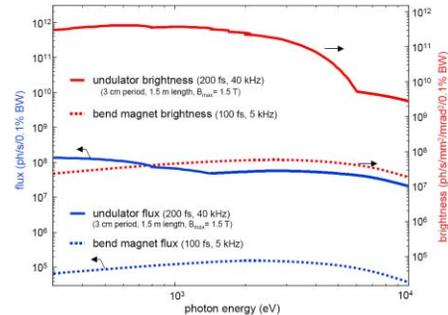
Figure 2: Flux and brightness of the original and upgraded fs slicing sources at the ALS.
