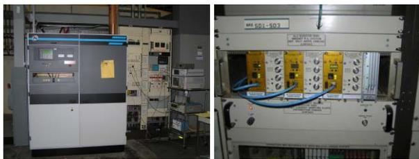
Figure 2: Example of newly installed hardware: New RF transmitter (IOT based); new controllers for small rsamped power supplies and rf amplitude (FPGA based).
