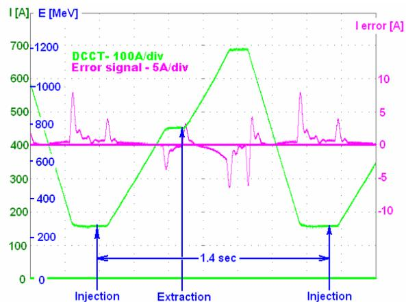
Figure 2: Booster operation cycle for one bunch mode.
