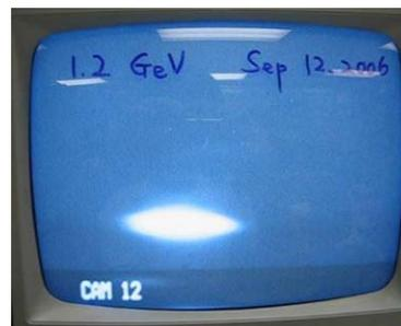
Figure 3: Synchrotron radiation image of the beam first ramped to 1.15 GeV.
