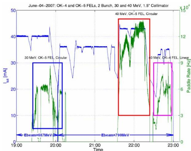
Figure 4: The first experience of the HIGS top-off operation in the electron loss mode gamma production with electron beam energies  $E=687$  and  $790$  MeV.
