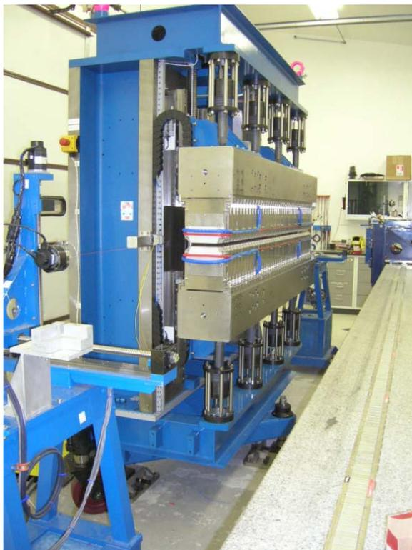
Figure 1: 100 mm Period Hybrid Wiggler
