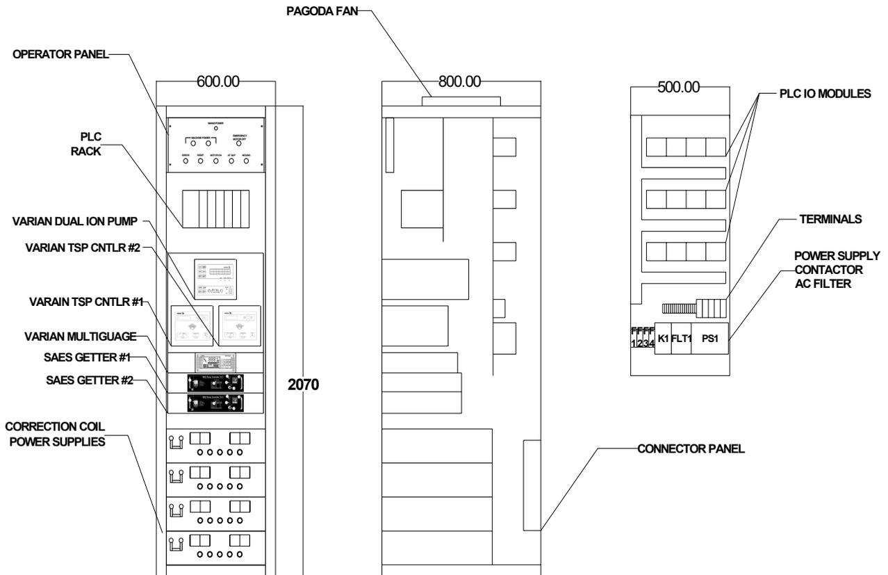
Figure 4: Controller layout
