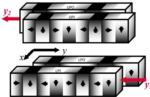
Figure 2: EPU helical plane
