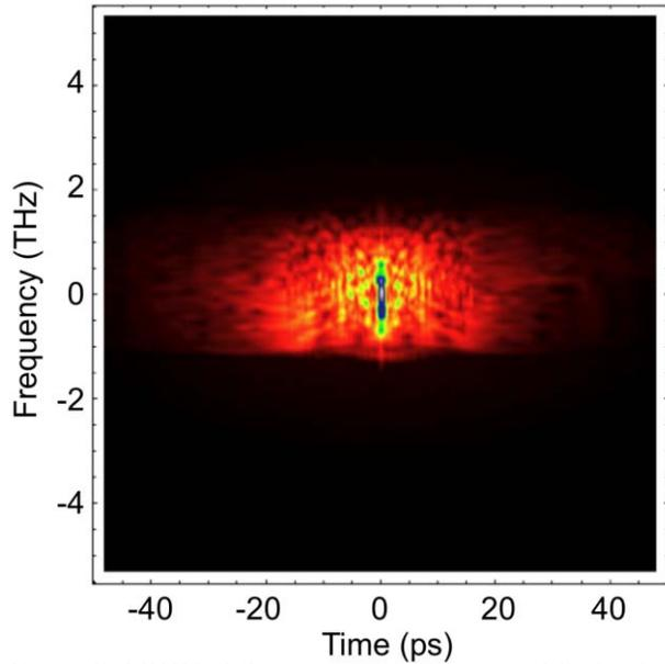
Figure 9: FROG of the compressed fiber-amplified pulse
