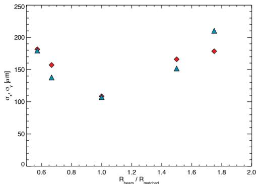
Figure 1: Dependence of the FEL spot size at the detector location on the mismatch of the electron, expressed by the beam radius as compared to the matched beam radius. Diamond and triangle markers refer to the size in the  $x$ - and  $y$ -plane, respectively.
