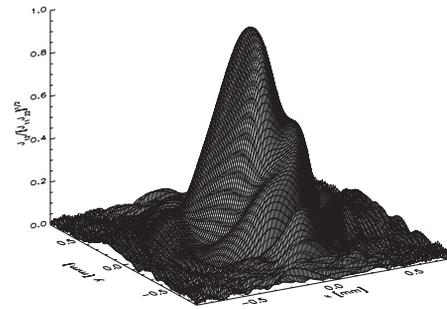
Figure 3: Complex coherence factor for LCLS for the start-end simulation, evaluated 115 m downstream of the undulator exit.
