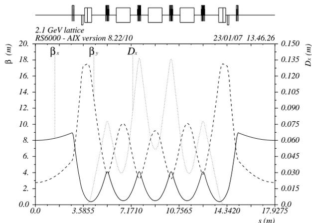
**Figure 1:** Lattice functions for one superperiod of the 2.1-GeV ring design.
