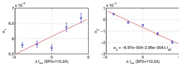
Figure 2: The first (left) and second (right) order alpha  $\alpha_2$  vs. SF.  $\alpha_1$  slightly depends on SF because of residual orbit offsets in sextupoles.
