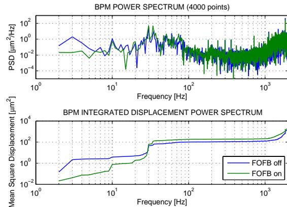
Figure 3: The power density of 4kHz BPM data corresponding to  $D_x = 0.5$  m with FOFB on or off. Data taken with 100 mA beam.
