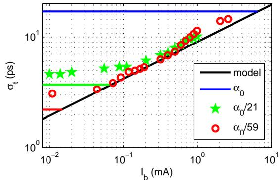
Figure 5: Measured bunch length in the two low alpha modes and the model calculation according to Ref. [8].
