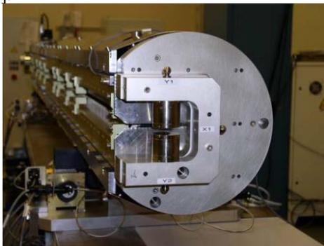
Figure 8: Magnets are placed on the ends of the undulator for the fiducialization.
