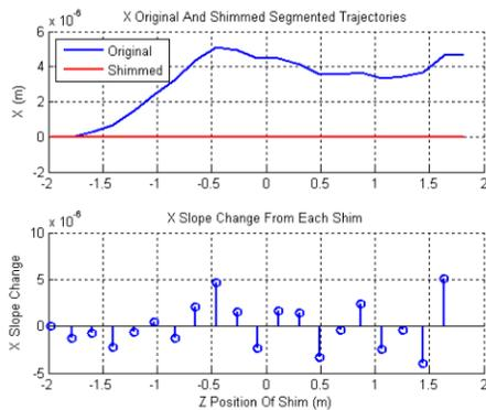
Figure 4: Slope change of each segment (bottom) which makes the trajectory straight (top).
