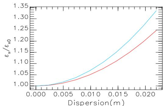
Figure 1: The horizontal emittance growth ratio as a function of external dispersion in the straights. The blue line is for the effective emittance, and the red line is for the horizontal emittance  $\epsilon_{x,0}$ .
