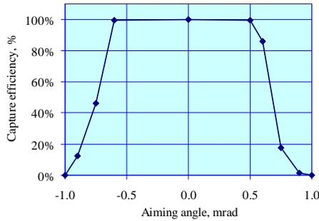
Fig. 1. Dependence of capture efficiency on the horizontal aiming angle of the injected beam.
