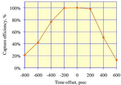
Fig. 5. Dependence of capture efficiency on the relative delay of the injected beam with respect to the stored beam.
