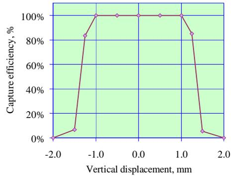
Fig. 4. Dependence of capture efficiency on the vertical position of the injected beam.
