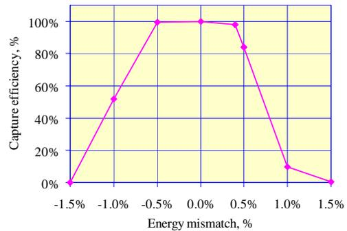
Fig. 6. Dependence of capture efficiency on the energy mismatch of the injected beam.
