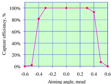
Fig. 3. Dependence of capture efficiency on the vertical aiming angle of the injected beam.
