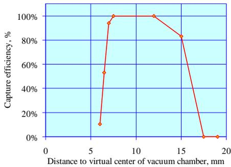
Fig. 2. Dependence of the capture efficiency on the distance between centers of the injected and stored beam. The particle with smaller separation are lost on the wall of the septum which is 6.4 mm away from the circulating beam.
