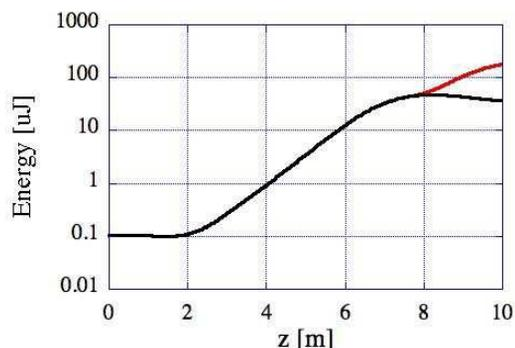
Figure 1: Simulation result of gain curves with taper (red) and without taper (black).
