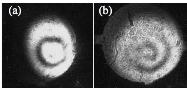
Figure 3: Multi-ring spatial structures in (a) SASE FEL and (b) seeded FEL.
