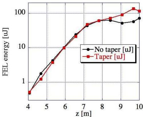
Figure 2: Experimental result of gain curves with taper (red) and without taper (black).
