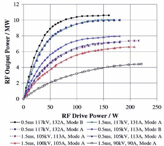
Figure 2: Transfer curves of the THALES TH1801 MBK.
