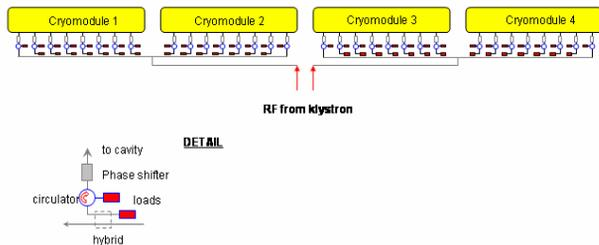
Figure 7: FLASH like waveguide distribution.
