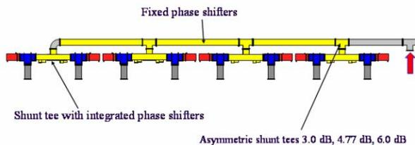
Figure 8: New combined waveguide distribution.
