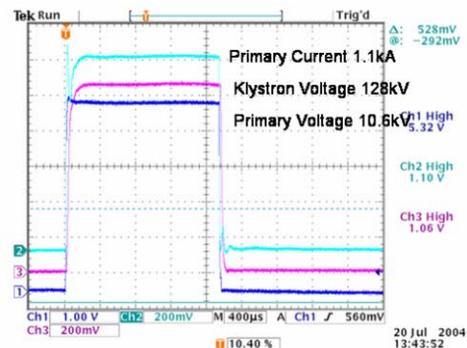
Figure 6: Waveforms measured with pulse cable between modulator and pulse transformer.
