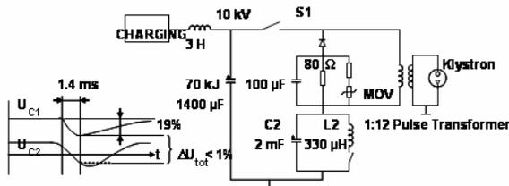
Figure 4: Schematic circuit diagram of the modulator.
