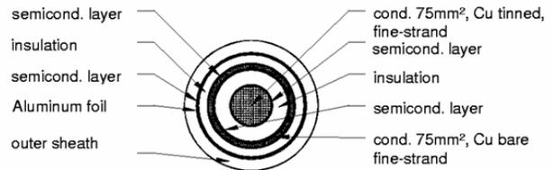
Figure 5: Cross section of the pulse cable.
