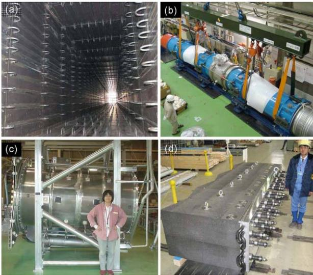
Figure 5: Photographs of the neutrino beam-line components (a) the decay volume (b) SCFM doublets (c) 3<sup>rd</sup> horn, and (d) a core unit of the hadron absorber.
