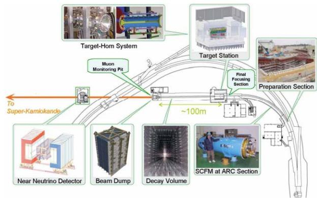
Figure 4: Schematic view of the neutrino beam-line.
