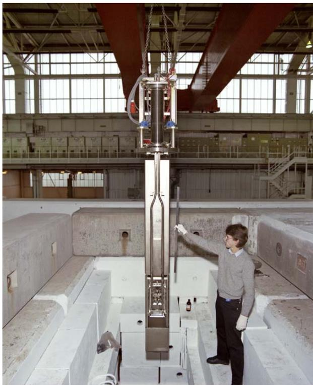
Figure 3: The intermediate target assembly — the ladder section is near the bottom of the assembly.
