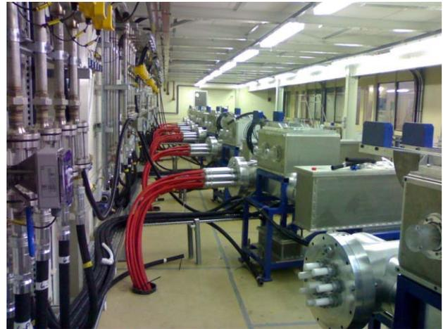
Figure 5: The new drivers for the fast kickers.
