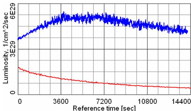
Figure 5: Cu-Cu luminosity for ion bunch intensity  $8 \times 10^9$  and 111 bunches. Average luminosity in 4 hour store  $4.6 \times 10^{29}$  and  $0.8 \times 10^{29}$   $\text{cm}^{-2}\text{s}^{-1}$  with (upper blue curve) and without (low red curve) electron cooling, respectively.
