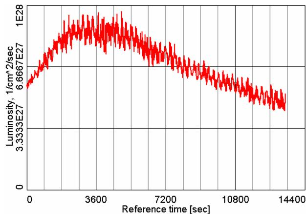
Figure 2: Electron cooling simulation of Au-Au luminosity: ion bunch intensity  $1 \times 10^9$ , 111 bunches; using single electron bunch per ion bunch. Average luminosity in 4 hour store is  $7 \times 10^{27} \text{ cm}^{-2} \text{ s}^{-1}$ .
