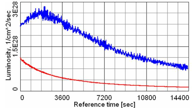
Figure 3: Simulation of Au-Au luminosity for ion bunch intensity  $2 \times 10^9$  and 111 bunches using two 5nC electron bunches per ion bunch with (blue top curve) and without (red bottom curve) electron cooling, taking  $\beta^* = 0.5 \text{ m}$  and 1 m, respectively.
