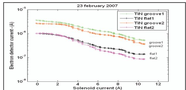
Figure 8. The collector current (not normalized to unit area) with external solenoid field ~20Gauss (at 11A).
