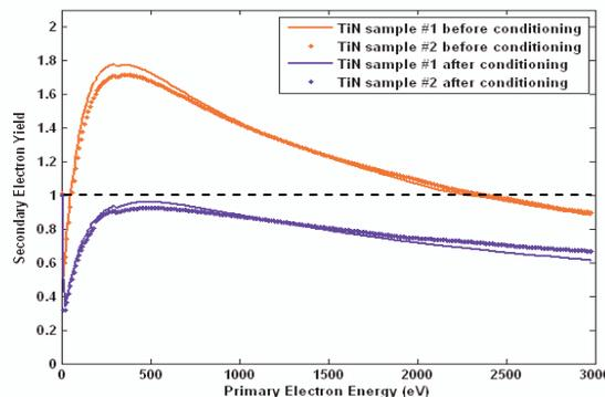
Figure 3. SEY before and after conditioning. TiN/Al samples were inserted in the PEP-II stainless steel chamber respectively in the plane of the synchrotron radiation fan (0° position) and out of this plane (45° position).
