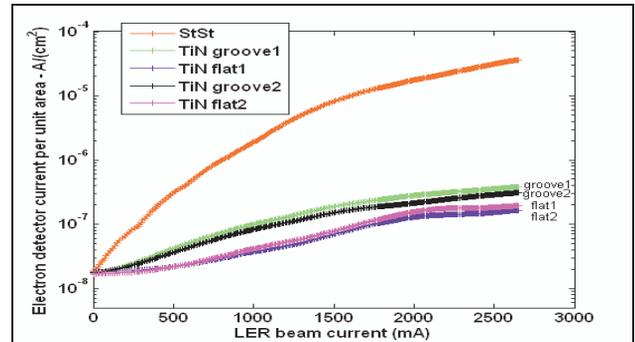
Figure 7. Experimental observation of the electron signal [A/cm<sup>2</sup>] in stainless steel, fin (groove) and flat chambers.
