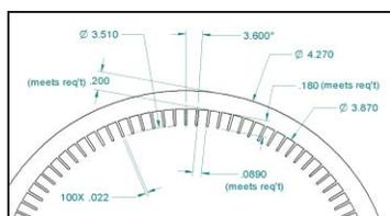
Figure 5. Fin chamber cross section and dimensions.
