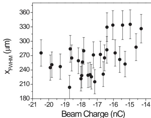
Figure 4: Dependence of the focused beam spot size on the beam charge under otherwise similar conditions.
