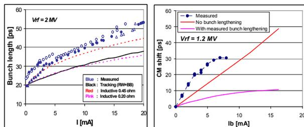
Figure 9: Bunch lengthening (left) and synchronous phase shift (right) measured with a streak camera.
