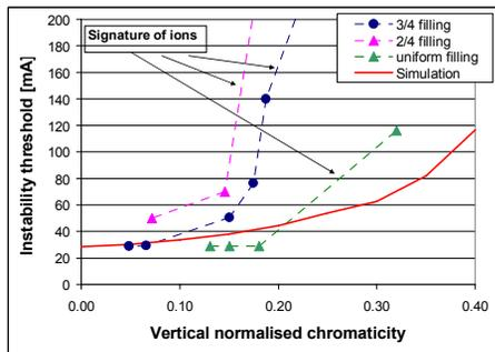
Figure1: Measured vertical multibunch instability threshold versus chromaticity.
