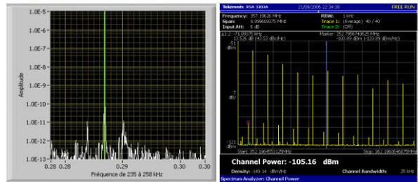
Figure 3: Observation of vertical  $m=-1$  mode excitation in 3/4<sup>th</sup> filling. Left: Display of relative head-tail modes. Right: Global spectrum.
