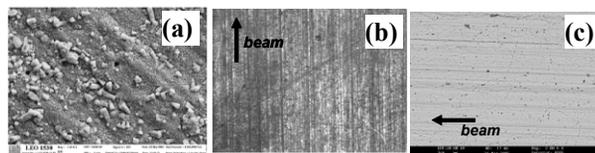
Figure 10: Surface of a NEG coated Al chamber (left) measured at the ESRF [4]. Surface of a SOLEIL Al chamber before (middle) and after (right) NEG coating.
