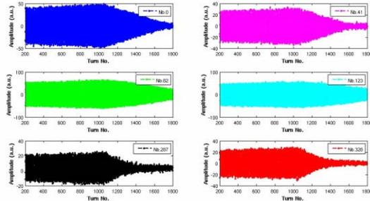
Figure 4: Observed envelopes of centre of mass bunch oscillations via transverse feedback.
