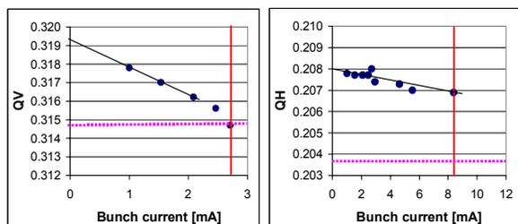
Figure 8: Measured dipole detuning. Left: Vertical. Right: Horizontal. Red line: TMCI threshold. Pink line: One synchrotron tune separation from the zero current tune.
