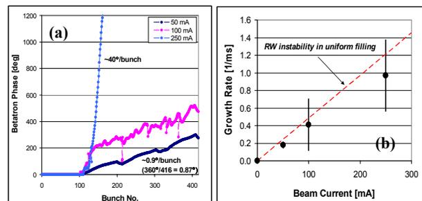
Figure 6: Left: Phase of vertical bunch oscillations measured at 50, 100 and 250 mA in 3/4<sup>th</sup> filling. Right: Measured average vertical growth rate versus beam current and that expected from RW instability.
