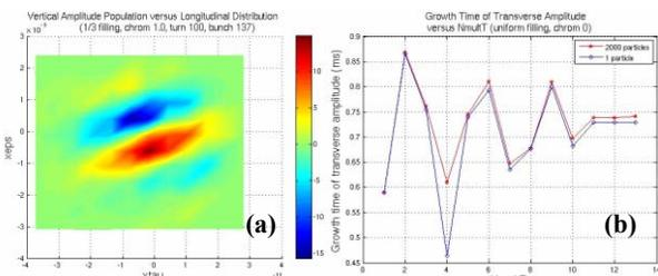
Figure 7: Impact of multi-turn effect on the instability growth rate (left) and bunch internal motion (right).
