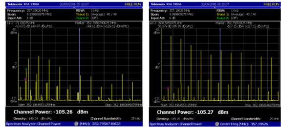
Figure 2: Spectra of vertically instable beam in 3/4<sup>th</sup> filling. Left: RW dominated. Right: Ion dominated.
