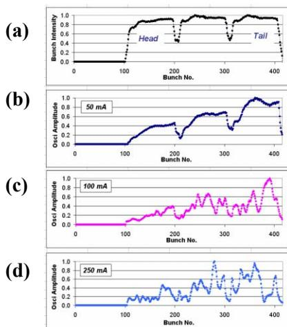
Figure 5: Measured vertical instability in 3/4<sup>th</sup> filling. Top: Current along a bunch train. Lower three: Oscillation amplitude versus bunch train at 50, 100 and 250 mA.
