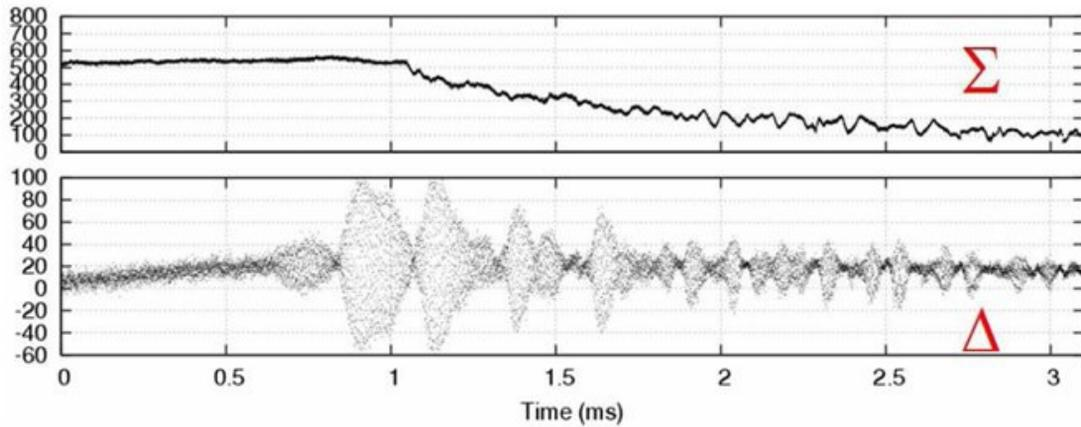
Figure 5: Comparison of the beam loss and tail slice oscillation for a 3.2 ms period before extraction. Upper graph: sum signal of the tail slice; bottom graph: difference signal of the tail slice, with arbitrary unit.
