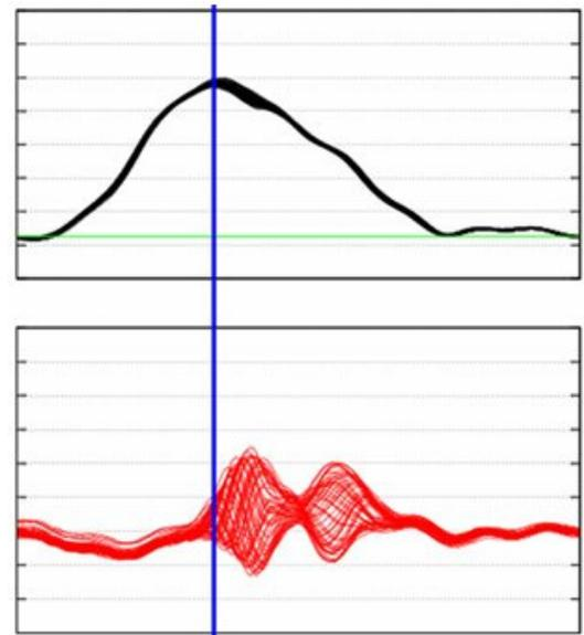
Figure 4: The centroid oscillations in the tail, mode 1.
