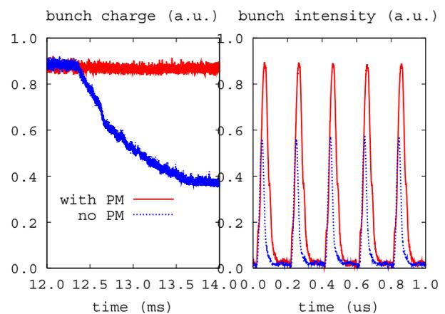
Figure 1: Beam loss observed with resistive wall monitor, phase modulation is used to suppress the instability.
