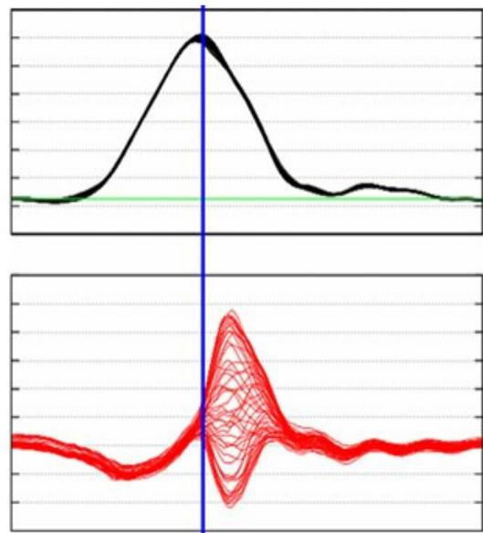
Figure 3: The centroid oscillations in the tail, mode 0. Upper graph: the sum of the top and bottom BPM signals; bottom graph: the difference of top and bottom BPM signals.
