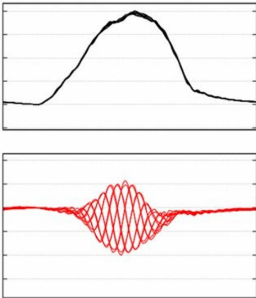
Figure 6: The centroid oscillations in head-tail instability induced in the RCS. Upper: the sum of BPM signals; bottom: the difference of the BPM signals.
