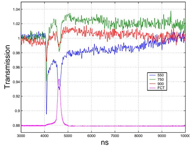
Figure 6: Transmission of the sapphire sample at various wavelengths during ion beam irradiation. Blue — transmission at 550 nm, red — 750 nm, green — 900 nm, magenta — temporal profile of heating beam in arb. units.
