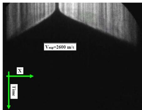
Figure 4: Expansion of a lead foil recorded by streak camera. Foil expansion rate estimated from the slope in this record is 2600 m/s.
