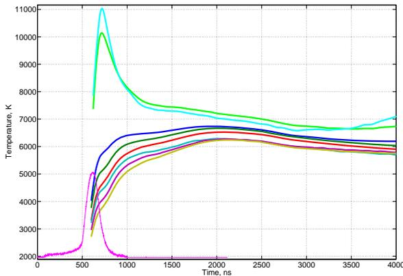
Figure 2: Temperature record of ion beam-heated tungsten foil. Blue, dark green, red, light blue, magenta, brown – brightness temperatures at 550 nm, 750 nm, 900 nm, 1100 nm, 1300 nm and 1500 nm respectively; green and cyan — fitted temperatures with grey and linear law of emissivity respectively [5]; light magenta — temporal profile of heating beam in arb. units.
