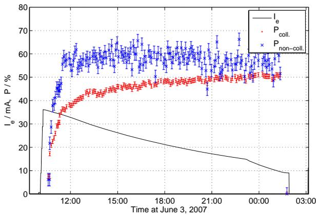
Figure 3: Positron current (—), polarization of colliding bunches (●) and non-colliding bunches (×) during a run.
