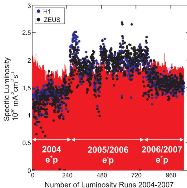
Figure 2: Measured specific luminosity of H1 and ZEUS (●) and theoretical prediction based on beam parameters (bars).
