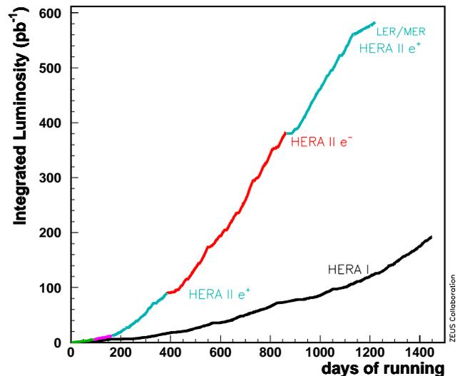
Figure 1: Delivered luminosity of HERA I and II.
