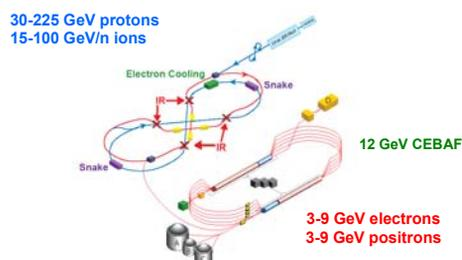
Figure 1: A schematic drawing of ELIC ring-ring design.
