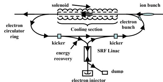
Figure 2: Layout of electron cooler for ELIC.
