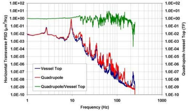
Figure 3: Displacement PSD of the vacuum vessel top versus the quadrupole in the horizontal transverse direction and its corresponding transfer function, on the CMTB; measured on 12 February 2007.
