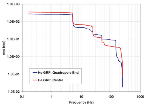
Figure 5: Integrated displacement PSD spectra inside He GRP in two positions along the module, quadrupole end and center in the horizontal transverse direction; measured on 24 July 2006.
