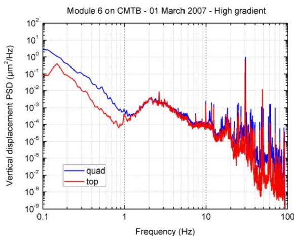
Figure 6: PSDs measured on vessel top and on quad during high power RF tests: the klystron was running at 10 Hz and the average gradient achieved was  $\sim 27 \text{ MV/m}$ .
