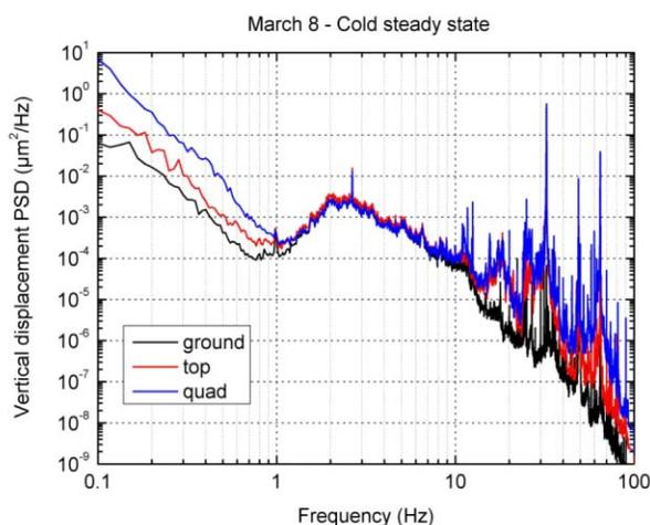
Figure 5: PSDs of ground, vessel top and quadrupole in cold steady state with RF off, measured just after reaching the cold stable conditions at the end of the 11<sup>th</sup> cooldown.
